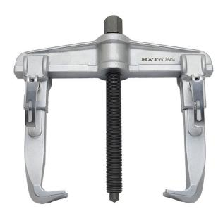
BATO Puller 160x150mm. 2-arms with metal clip lock for quick adjustment. Puller can be 65-150mm internally and 115-210mm externally.
