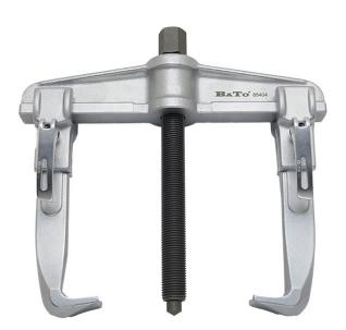
BATO Puller 90x100mm. 2-arms with metal clip lock for quick adjustment. Puller can be 40-90mm internally and 80-130mm externally.
